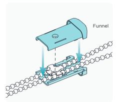
**3.** Slide the Shield through the chain and over the funnels.
