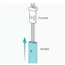
**4.** Install binding posts at the top and bottom of the funnels.
